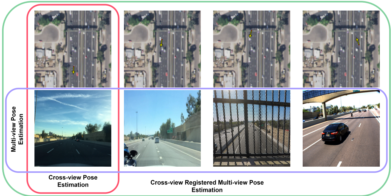
Figure 1. Most camera pose estimation work either specifically looks at cross-view pose estimation with a single aerial/ground image pair or multi-view pose estimation with imagery of all the same form. In this work, we explore extending to the joint setting of multi-view ground imagery within a reference aerial image.
